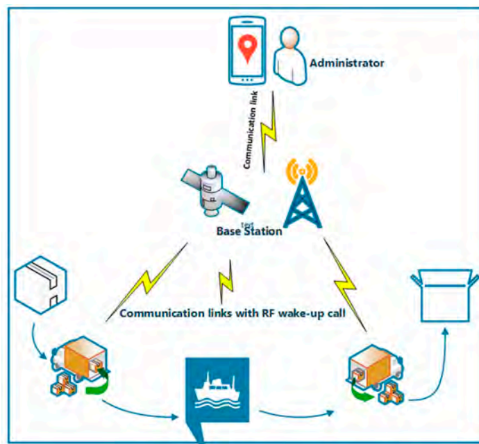
Figure 11. Description of passive wake-up radio for asset tracking application.
